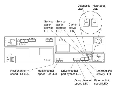
Figure 69. LEDs, controls, and connectors of controllers with two standard Fibre Channel host expansion channels
